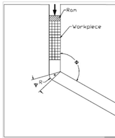
Fig. 4: A section through the ECAP die.
