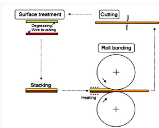
**Fig. 1:** Schematic showing the accumulative roll bonding process.
